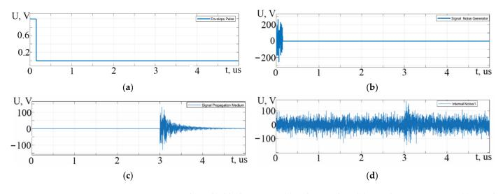
**Figure 3.** Signals at the blocks output: (**a**) pulse envelop; (**b**) signal noise generator; (**c**) signal propagation medium; and (**d**) internal noise.
