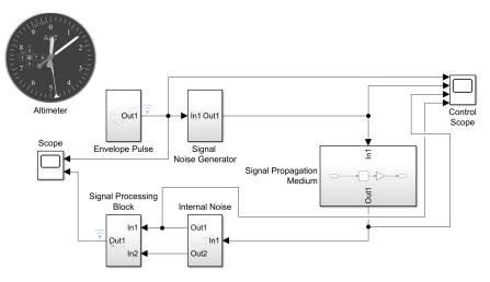
**Figure 2.** A simulation model of a wideband altimeter containing a transceiver part and realizing signal distortion during its propagation in the environment and reflection from the underlying surface.
