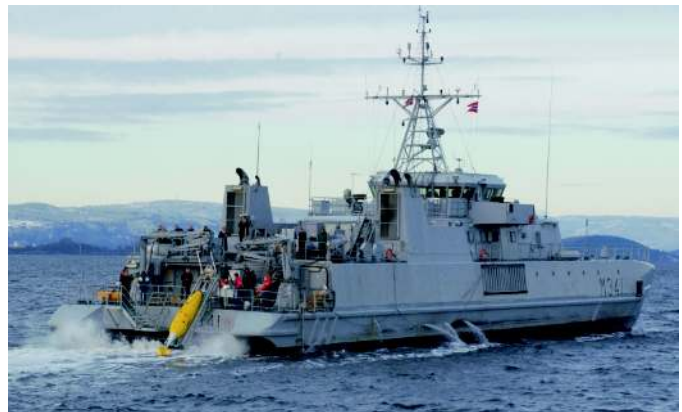
Fig. 1. The HUGIN AUV immediately before launch from the RNoN mine hunter KNM Karmøy in December 2001.
