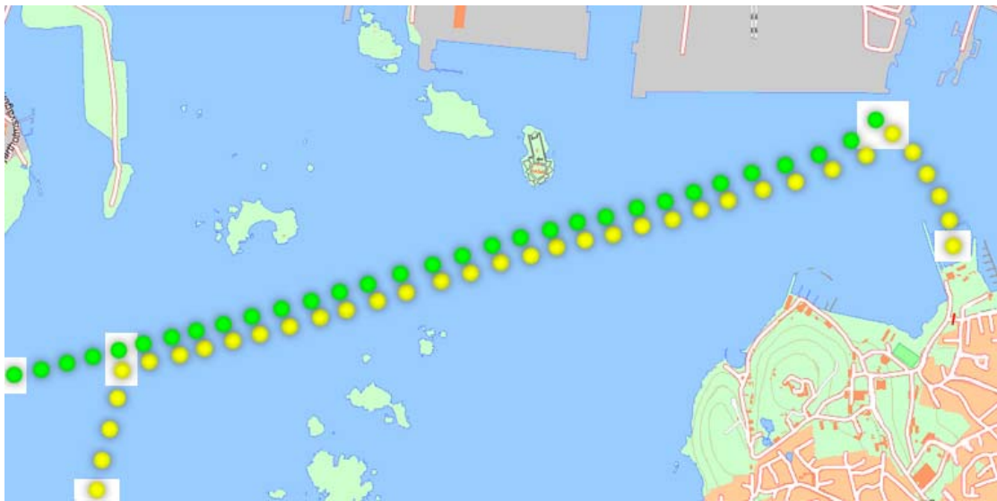
Figure 5.12 A pilot-boat scenario detected from AIS-data.
