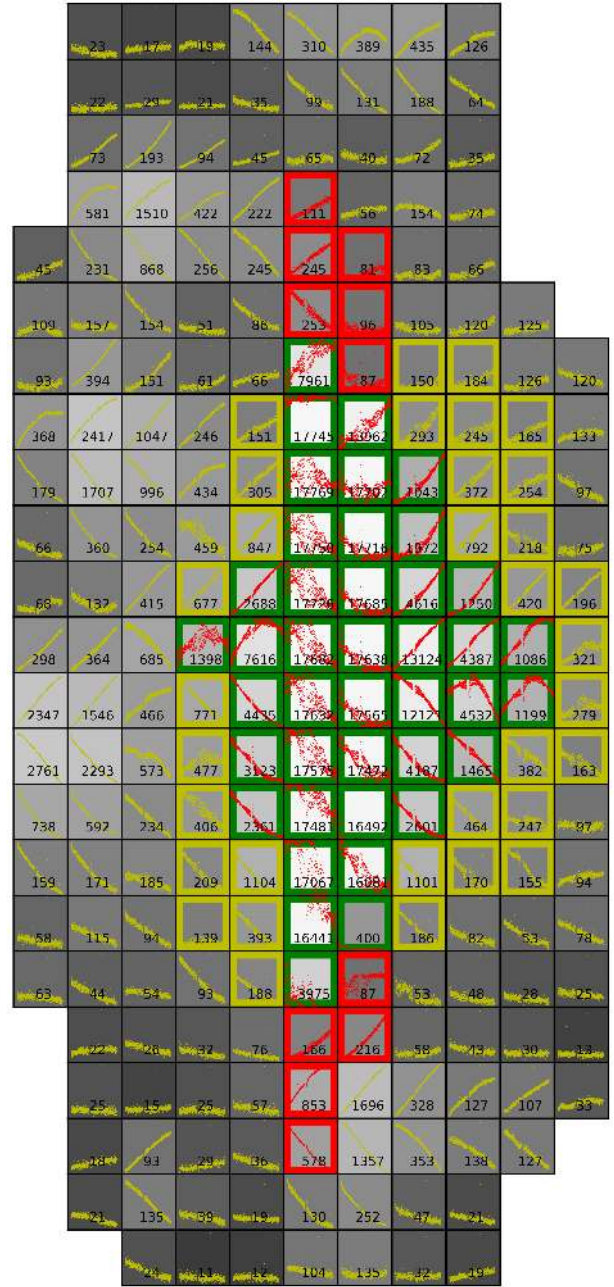
Fig. 9. Custom pixel mask for the Q8 data of KIC 4930889. Individual pixel-level light curves are plotted for each pixel that was downloaded from the spacecraft. The numerical values and the background colour indicate the flux levels in each pixel. The pixels with green and red borders were used to extract the standard Kepler light curves. We added yellow pixels (significant signal is present) and removed red pixels (non-significant signal or contamination from nearby stars) in our custom mask for the light curve extraction. This results in a light curve with significantly less instrumental effects and/or contamination than the standard extraction.
