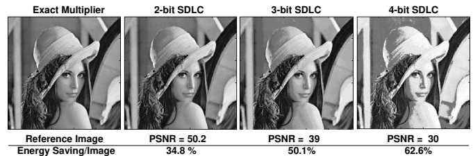
Fig. 13. Output quality after applying Gaussian blur filtering for different degrees of logic compression of the proposed (8 \times 8) multiplier.
