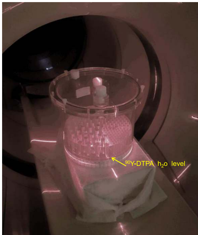
Fig. 1 Jaszczak deluxe phantom set in vertical position on a 20-cm-thick paper bloc modelling the conventional attenuation as only a part of the hot rod insert was filled with active solution in order to reach a typical clinical liver absorbed dose in selective liver ^{90}\text{Y} radioembolization
