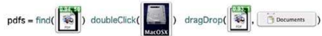
Figure 1: Sikuli Search allows users to search documentation and save custom annotations for a GUI element using its screenshot (captured by stretching a rectangle around it). Sikuli Script allows users to automate GUI interactions also using screenshots.
