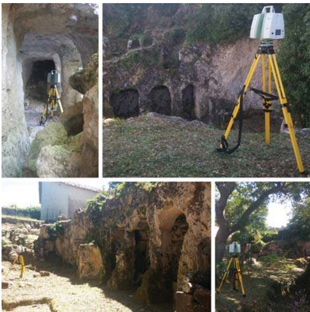
Fig.9: Survey operations with Leica Scan Station C10.
