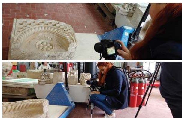
Fig.12: Photographic surveying: photogram acquisition operations.
