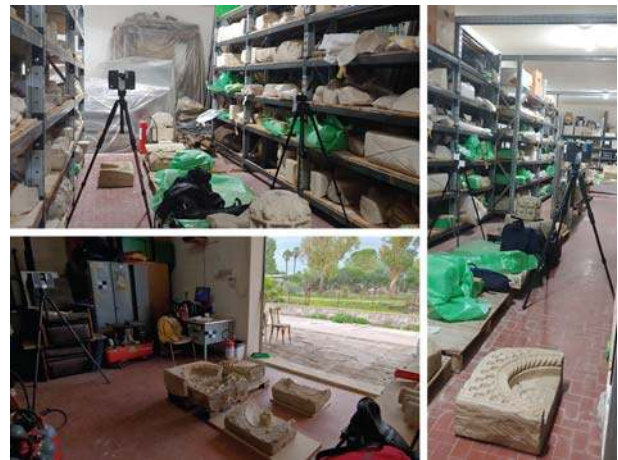
Fig.10: Survey operations with Faro CAM2 Focus: stores of Galleria Regionale of Palazzo Bellomo.
