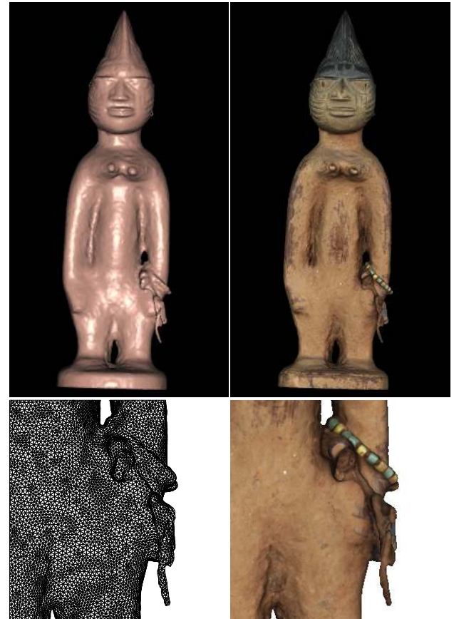
Figure 4. African model after convergence (57639 vertices). Top left: Gouraud shading. Top right: same view with texture mapping. Bottom: Detail of the model after convergence.
