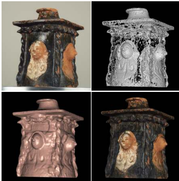
Figure 6. Example of a reconstruction with bad image correlations. Top left: one of the original images. Top right: rendering of the correlation voting volume. Bottom left: snake mesh after convergence. Bottom right: textured mesh.
