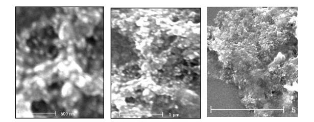
silica nanostructure was observed. The results of this project could be useful for the development of new routes towards the environmentally benign synthesis and patterning of well defined silicon based material at low cost.
