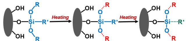
FIGURE 7. Mechanism of thermal degradation of a silane grafted on silica. (During heating, the unreacted alkoxy groups marked in red will leave firstly; with further increasing temperature, the Si-R' bond of the side chain from the silane marked in green will be broken).
