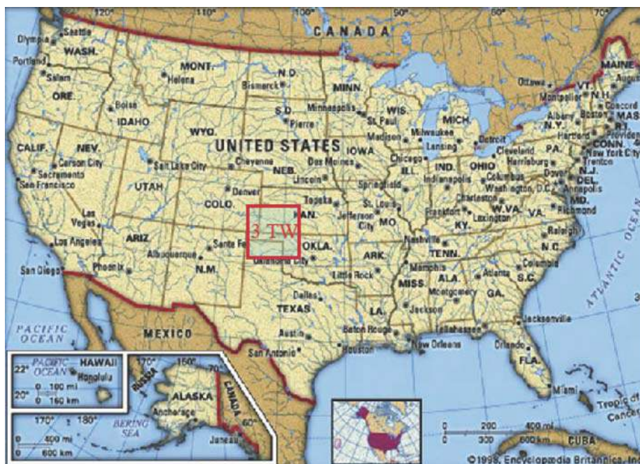
Figure 1. The red square shows the amount of land needed for a solar farm operating at 10% efficiency to match the 3 TW of power currently consumed in the United States. 2
