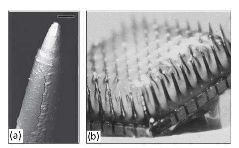
**Figure 17.** In vivo failures common in today's heterogeneously integrated silicon-based neural probes. The Utah intracortical electrode array (Blackrock). (a) Side view of an electrode with a large longitudinal crack in the parylene-C insulation adjacent to surface irregularities (20  $\mu$ m scale). (b) Explanted UIEA array at 10 months. The array was completely encapsulated. Reproduced with permission from Bernardin ©2018 [50].
