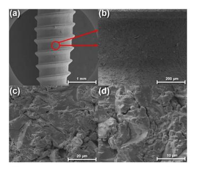
**Figure 15.** Scanning electron microscope images of a SiC-coated titanium implant at various magnifications. Image (**a**) shows the overall surface of the implant, whereas images (**b**–**d**) show detailed images of the implant surface morphology at increasing magnifications [47].
