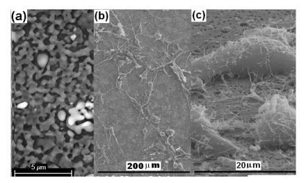
**Figure 14.** SEM micrograph (**a**) of 1.4  $\mu$ m of HA film on ~16 nm np-SiC obtained after thermal treatment at ~900 °C for 12 h. (**b**) MG-63 cell attachment to 1.4  $\mu$ m thick HA on ~16 nm np-SiC at lower magnification and (**c**) higher magnification [2].
