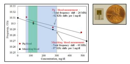
**Figure 9.** Measured relative resonance frequency shift dependence on glucose concentration. Photograph of the RF patch antenna on 4H-SiC. Note fairly linear response vs. glucose concentration [3].
