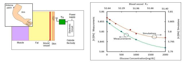
**Figure 10.** Non-invasive glucose sensing antenna configuration (**left**) on top of the arm to detect glucose changes in the cephalic vein (inset) along with HFSS<sup>™</sup> simulation geometry. Measured vs. simulated data (**right**) using a tissue phantom, indicating that non-invasive glucose detection is possible with the remote antenna configuration [21].
