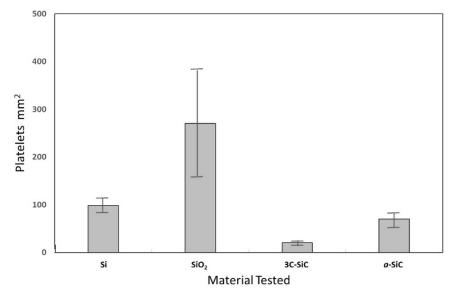
**Figure 3.** Dynamic hemocompatibility histogram of platelet activation of Si and SiO<sub>2</sub> on Si and 3C-SiC, as well as *a*-SiC on Si, and using standard deviation as the error bar. Activated platelets per mm<sup>2</sup> were used to evaluate the hemocompatibility of the materials. Test coupons:  $50 \times 75 \text{ mm}^2$  [3].
