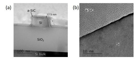
**Figure 12.** Si/SiC nanowire DNA sensor structure. (**a**) TEM cross-section image of a Si NW etched from SOI substrate and covered with *a*-SiC deposited by PECVD, and (**b**) HR-TEM image at the Si/*a*-SiC interface [43].
