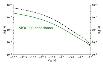
**Figure 13.** Transfer characteristics of backgated core-shell Si/*a*-SiC nanoribbon devices: *a*-SiC-coated SOI device resulting in thin SiC shell. Drain current plotted with solid line and gate current with dashed line [43].
