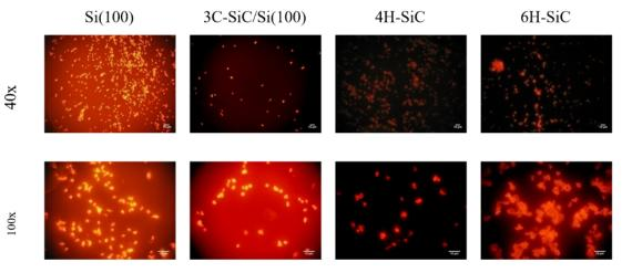
**Figure 2.** Static hemocompatibility study. Fluorescent micrographs comparing adhered platelets on three different SiC polytypes and Si. 3C-SiC clearly shows lower adhesion and high circularity while Si presented the highest adhesion. 4H and 6H-SiC evidenced the presence of clumps and a high degree of activation [2].
