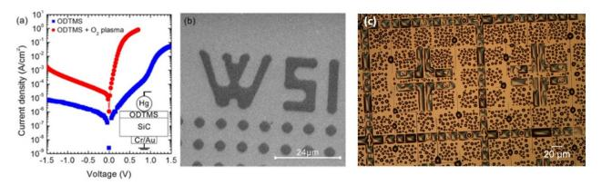
**Figure 6.** SAM synthesis (ODTMS-functionalized) on 6H-SiC. (**a**) IV curves and (**b**) SEM micrograph of regions with different electrical conductivities. Dark areas indicate oxygen plasma-treated regions. (**c**) Wettability image of micropatterned ODTMS-modified SiC surface. Note water droplets condense preferentially in hydrophilic oxygen plasma-exposed regions [2].
