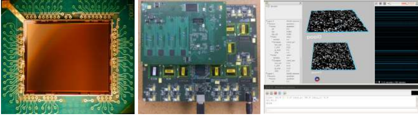
Fig. 2. Neurogrid. Spiking neural networks with up to 16 layers, each with up to 256 \times 256 neurons, are modeled with sixteen 12 \times 14 sq-mm Neurocores ( left ) assembled on a 6.5 \times 7.5 sq-in circuit board ( center , main board). Neurocores, connected in a binary tree with 91M spikes/s links (peak rate), relay their spikes to a routing table ( center , daughterboard) that supports programmable weighted connections. Spike activity is visualized in real time ( right ). The entire 1M-neuron system consumes 3.1W.
