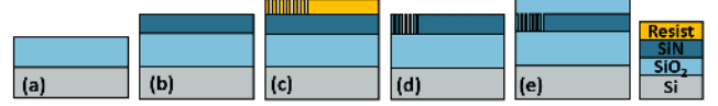
Fig. 2. Device fabrication process: (a) silicon substrate with 2-3 \mu m of thermal SiO_2 , (b) PECVD SiN deposition, (c) Lithography, (d) SiN ICP etching with SF_6:CHF_3 , and (e) 1 \mu m PECVD SiO_2 deposition.
