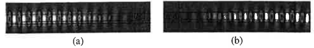
Fig. 2. Top view field plots of the polarization rotator, obtained using a fully vectorial eigenmode expansion tool. (a) E_x field (TE polarization). (b) E_y field (TM polarization).
