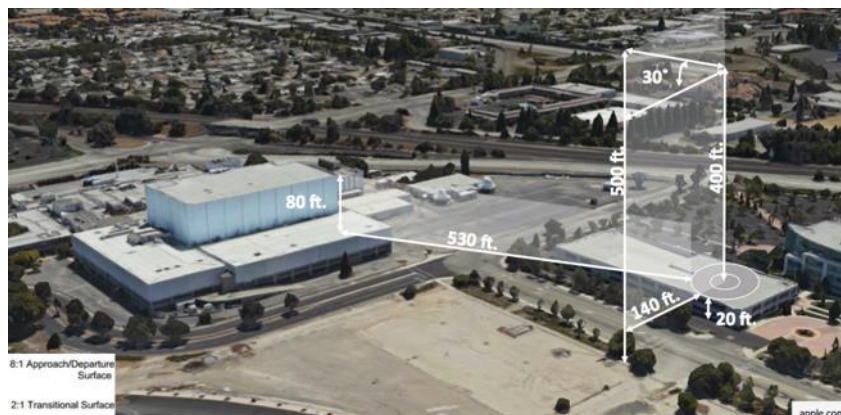
Figure 9. Private helipad approach/departure path example
