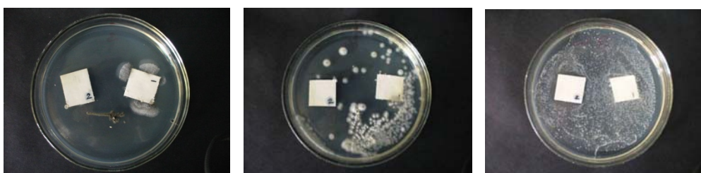
Fig. 3. Growth of A. pullulans (left), P. phoeniceum (middle), and S. aureus (right) cultures on pasteboard samples modified by silver nanoparticles (note, the white spots correspond to microbial colonies). Sample #1 is a control sample, i.e., it was covered with nonmodified paint; sample #2 was covered with the paint modified by silver nanoparticles at a density of 0.8 µg/cm 2
