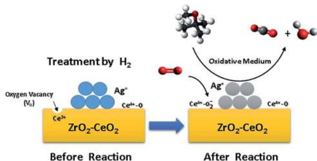
Fig. 10 Scheme proposed to explain the effect of the partial reduction of ceria on metallic silver to destroy MTBE by CWAO.
