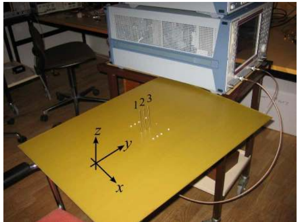
Fig. 5. Monopole uniform linear array of three elements, with the coordinate system used in the radiation pattern measurement.
