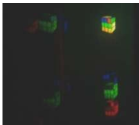
Fig. 5. Higher diffraction orders visible on the projection screen.
