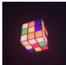
Fig. 4. (Media 1) Experimental projection showing the faint background non-diffracted light.
