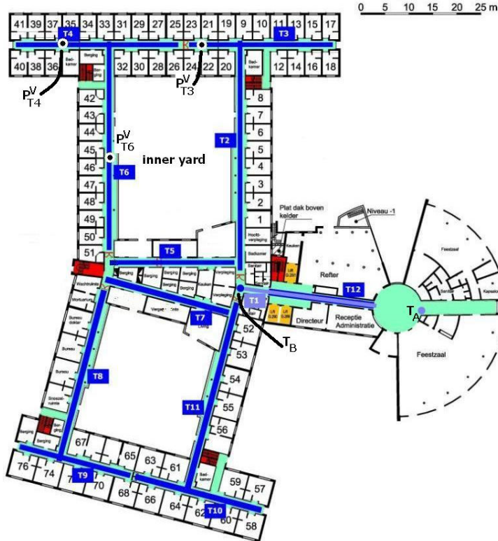
Fig. 2 Ground plan of 'De Vijvers' with indication of transmitters T_A and T_B and the measurement trajectories T1-T12. The points for which the different path loss contributions are investigated in Table 3 are indicated on T3, T4, and T6 with a black dot within a white dot.
