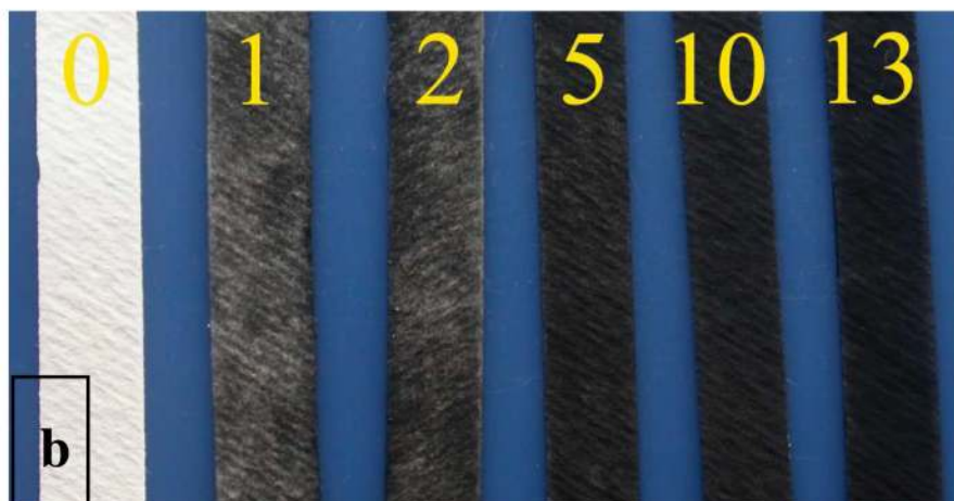
Figure 1. (A) Chemical structure of MC-LR. (B) Optical photographs of the SWNT-impregnated filter paper with a different number of the deposition cycles.
