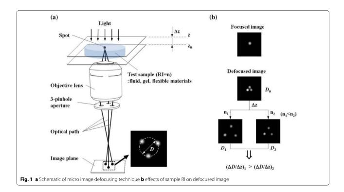
the multiple-pinhole aperture, which is attached directly behind an objective lens, and which divides the optical ray into three different optical paths via the pinholes. As shown in Fig. 1a, when a spot is not placed on the focal plane, three duplicated and separated spot images are produced on the image plane due to the optical path separation, while a single image of the spot is formed on the image plane when the spot is located on the focal plane.
