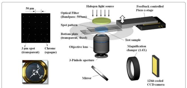
**Fig. 3** Experimental setup; the 3-pinhole aperture has 1.5 mm diameter pinholes (*d*) and 4 mm of the pinhole space (*d*'). The 10 nm resolution z-stage with the 3 μm-spot patterned plate is mounted on the microscope
