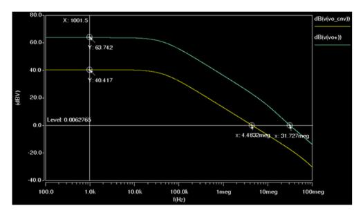
Figure 3. AC open-loop response in 45 nm.
