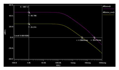
Figure 2. AC open-loop response in 22 nm.
