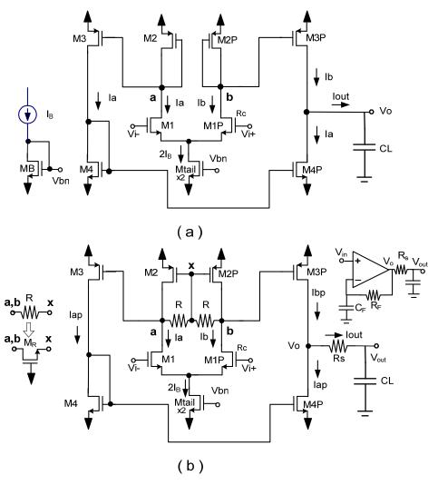
**Figure 1.** (a) Conventional one-stage op-amp without cascoding transistors. (b) One-stage op-amp with resistive local common mode feedback.
