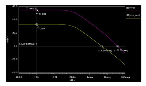
Figure 4. AC open-loop response in 90 nm.
