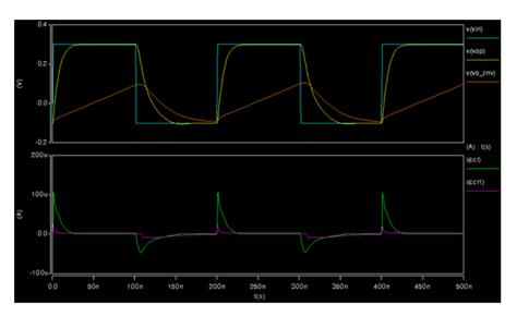
Figure 12. Transient simulation in 90 nm.
