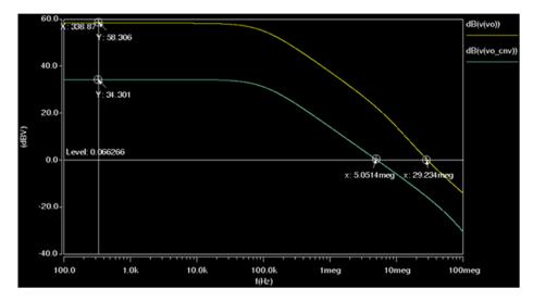
Figure 5. AC open-loop response in 180 nm.
