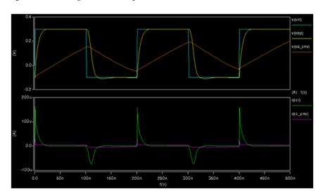
Figure 10. Transient simulation in 22 nm.
