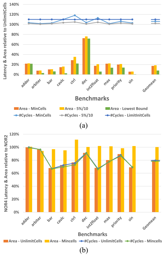
Fig. 8. Results of EPFL benchmarks for (a) NOR2 and (b) NOR4 as compared to NOR2.
