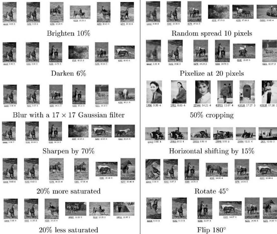
Fig. 16. The robustness of the system to image alterations. Due to space, only the best five matches are shown. The first image in each example is the query image. Database size: 200,000 images.
