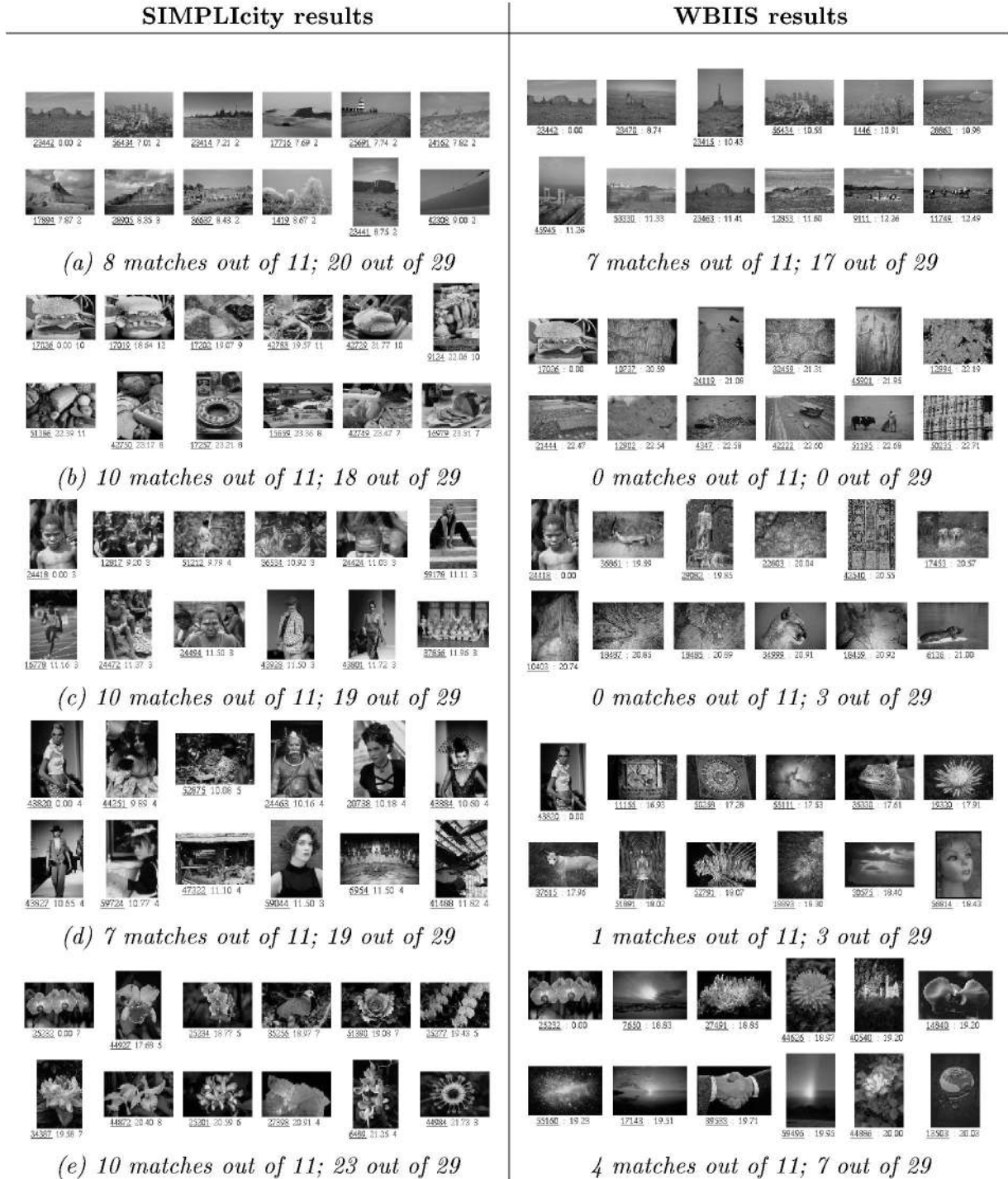
Fig. 11. Comparison of SIMPLicity and WBIIS. The query image is the upper-left corner image of each block of images. Due to the limitation of space, we show only two rows of images with the top 11 matches to each query. More matches can be viewed from the online demonstration site. (a) Natural out-door scene, (b) food, (c) people, (d) portrait, and (e) flower.
