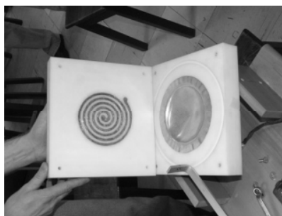
Figure 5. Die of electromagnetic forming device.
