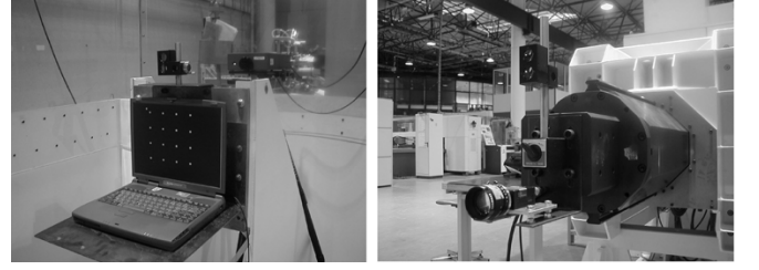
Fig. 5. Setup of the vision-based metrology evaluation. Left (fixed): an LCD target, a laser interferometer station, and its beam splitter block. Right (in motion): a CCD camera and the laser retroreflective block.
