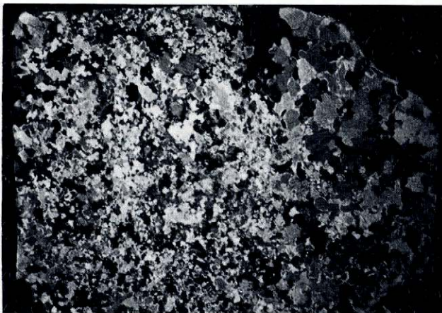
Fig. 12. Ice fabric from the February 1973 experiment; tap-water ice deformed for 200 h.
