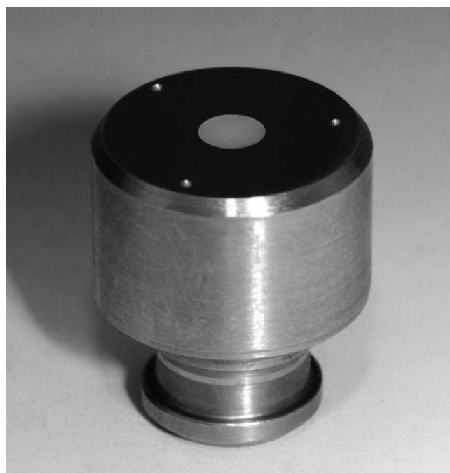
Figure 1. Custom stainless-steel fixture for generalized (bulk) wear.
