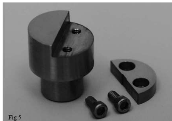
Figure 4. Slit (gap) fixture for generalized wear simulation.
