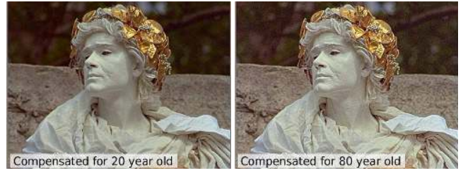
Figure 12: Image compensated for viewing on a 10 \text{ cd/m}^2 peak luminance display, individually for younger and older observers. Enlarge to see the difference.
