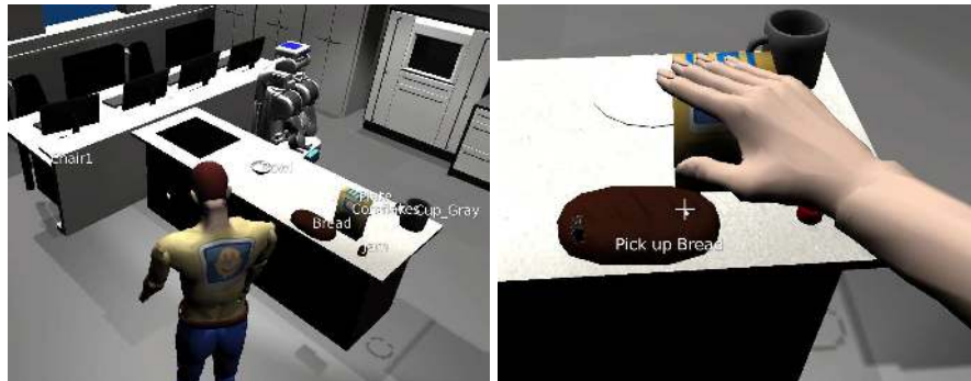
Fig. 3: Left: third-person view of the human component that is used to navigate in the environment, displaying the names of objects that the human can interact with. Right: first-person perspective of the human avatar that indicates a possible “pick-up-action” with the bread.
