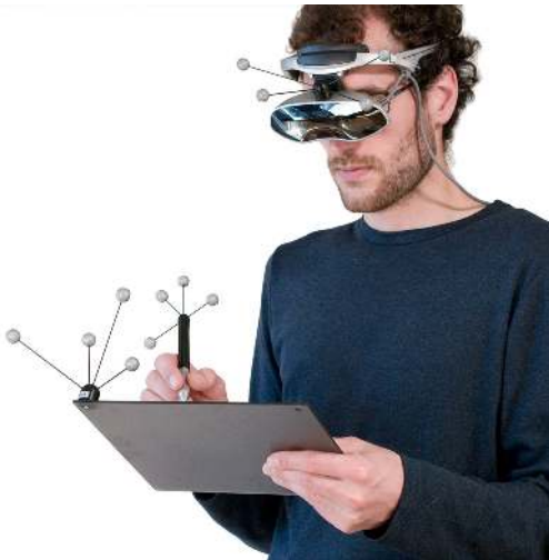
Figure 3: Each user is equipped with input devices pen and PIP and a head mounted display when interacting with PhysicsPlayground.
