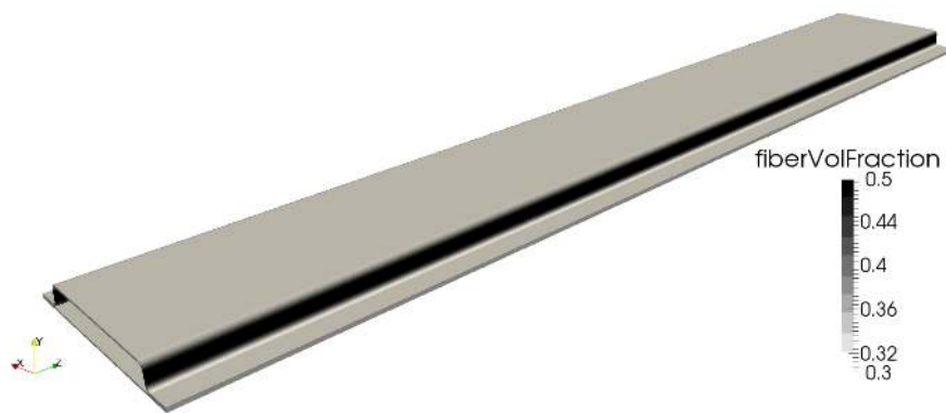
Figure 14. Fiber volume fraction of the sandwich part at the beginning of the simulation.
