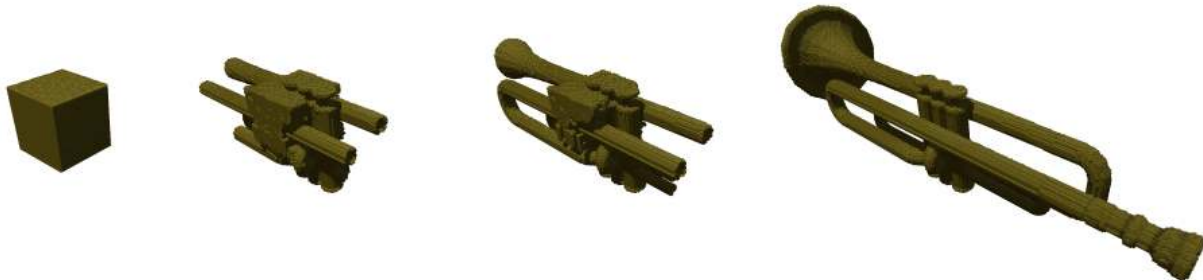
Fig. 3. An ensemble of catoms transforming from a solid cube into a trumpet using a distributed metamodule-based shape change algorithm. This ensemble includes in excess of 165,000 modules. A complete video is available at http://www.cs.cmu.edu/~claytronics/movies/trumpet-1920x1200.mp4 . This simulation is at the limit of what can be done with the original DPRSim, and requires over three weeks of processing time with physics disabled.
