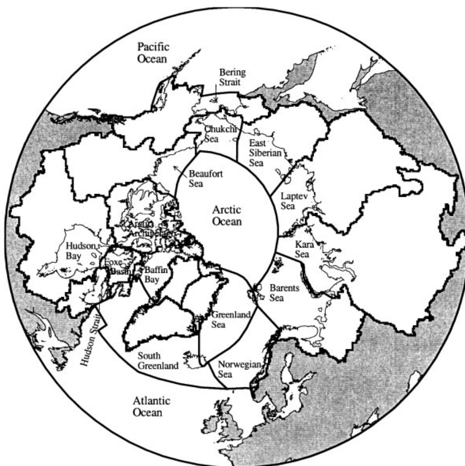
Figure 1. Pan-Arctic domain by sea basin boundaries. Basin boundaries are derived from a digital river network at 30' grid-cell resolution (Vörösmarty et al. , 2000a). Shaded region represents areas outside of the pan-Arctic drainage system
