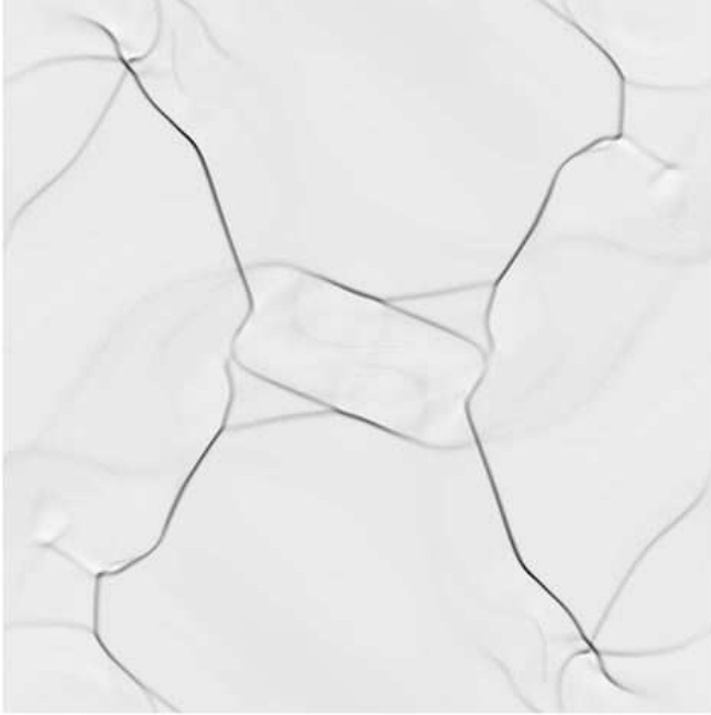
FIG. 20.— Orszag-Tang vortex: \nabla \cdot \mathbf{v} at t = 0.48 seconds for the 512^2 zone calculation.
