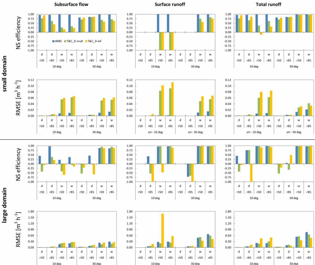
Figure 7 | Quantification of the agreement between runoff simulated by HYDRUS-3D and the flow-approximation based models using the NSE and the RMSE.
