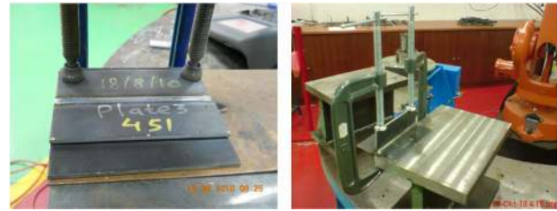
Fig. 2. Clamping conditions for butt and T-joints.
