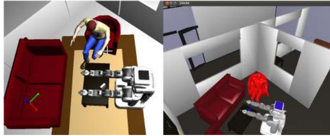
Fig. 2. On the left side, the MORSE environment ; on the right side, the same environment, as perceived by the robot in the SPARK situation assessment module.
