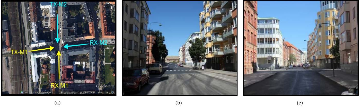
Fig. 1. (a) Google Earth TM [15] aerial image of the investigated urban crossroads scenario in the city of Lund with two vehicles moving towards the intersection at a speed of approximately 10 m/s (N55° 42' 37'', E13° 11' 15''). (b) and (c) show the perspective from the receiving vehicle RX-M1 and TX-M1, respectively.
