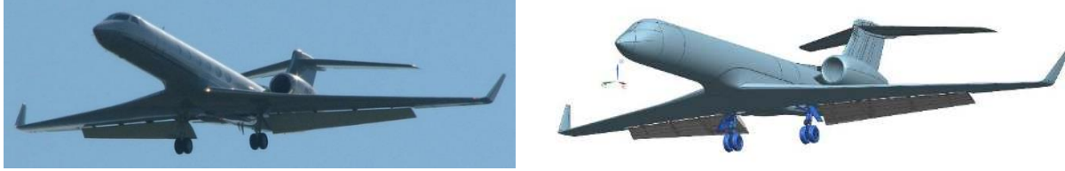
c) 39° deflected flap with main gear deployed, left image 2006 flight test, right image simulated CAD model
