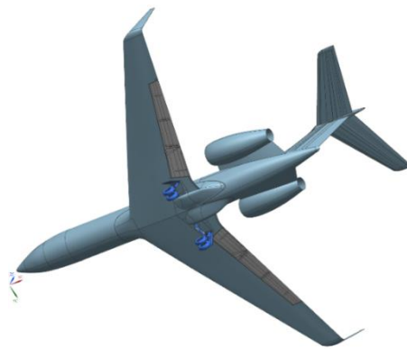
b) 0° flap (cruise wing) with main gear deployed, left image 2006 flight test, right image simulated CAD model
