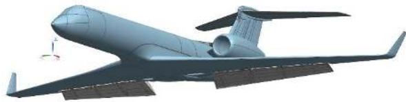
a) 39° deflected flap with main gear retracted, left image 2006 flight test, right image simulated CAD model
