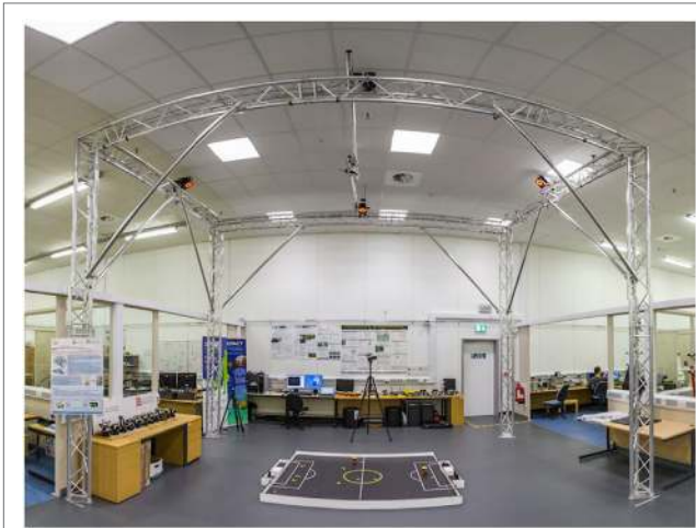
FIGURE 9 | Experimental infrastructure showing the arena on the bottom, the camera used to document the experiments, and the Vicon motion capturing system overhead.
