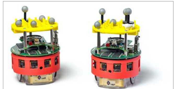
FIGURE 10 | Two e-puck robots with markers and IR sensors. The e-puck with Linux board fitted in between the e-puck motherboard (lower) and the e-puck speaker board (upper). Note the yellow “hat,” which provides a matrix of pins for the reflective marker spheres, which allow the tracking system to identify and track each robot.
