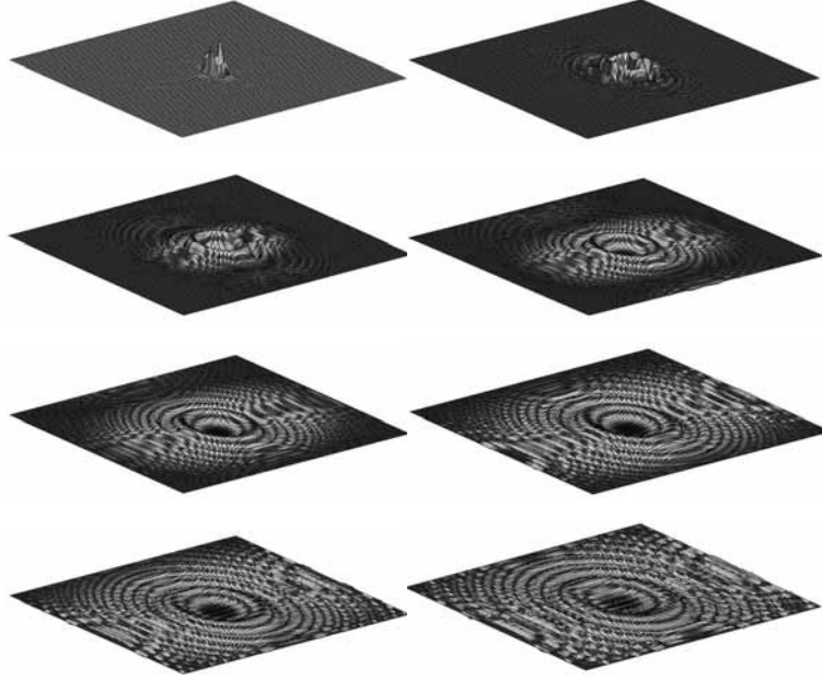
Fig. 5. Wave propagation at 10, 60, 110, 160, 210, 260, 310, 360 micro-sec due to center actuation by a PZT patch with an impulse moment excitation.
