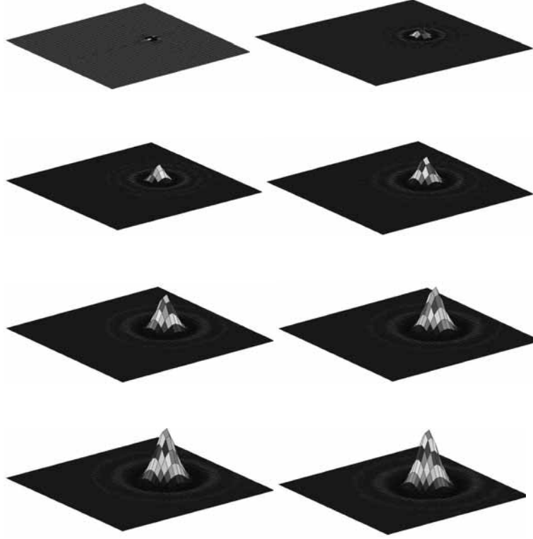
Fig. 4. Acoustic Wave propagation at 10, 60, 110, 160, 210, 260, 310, 360 micro-sec due to a lead break excitation modeled as a step input function.
