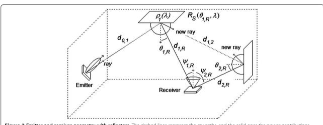
Figure 2 Emitter and receiver geometry with reflectors. The dashed lines represent the ray paths, and the solid ones the power contributions.
