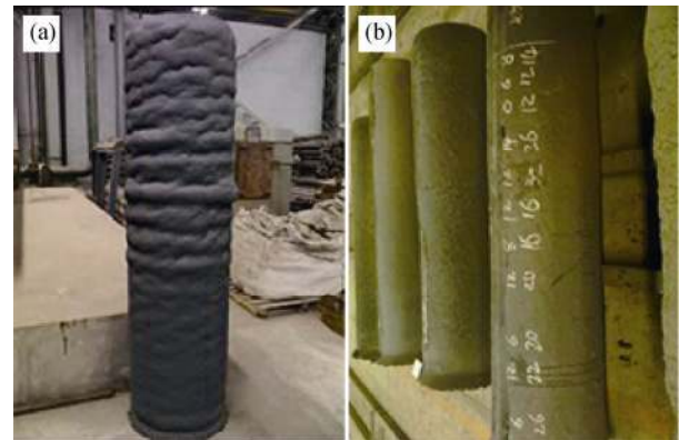
Fig. 14. Spray-formed high-speed steel billets with different superheat degrees ( R = 0.55 , v_{gi} = 300 \text{ m/s} , and Z = 0.5 \text{ m} ): (a) \Delta T = 150 \text{ K} ; (b) \Delta T = 100 \text{ K} .
