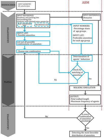
Figure 1. Flowchart of data between different plug-ins within the software (Source: Authors, 2020)
