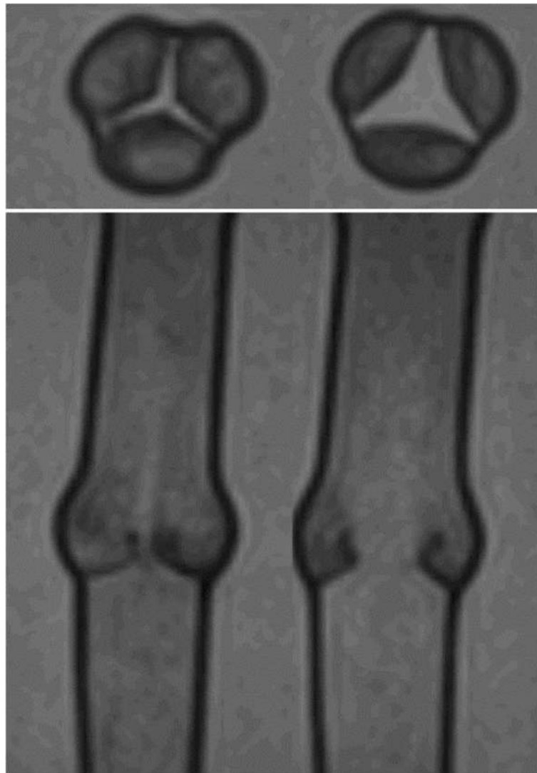
Fig. 6 Cine MRI images showing aortic valve phantom in simulated systole in short and long axis planes. Left image shows the valve leaflets closed. Right image shows leaflets open. (Corresponding video files attached – Additional file 2: Video S2)
