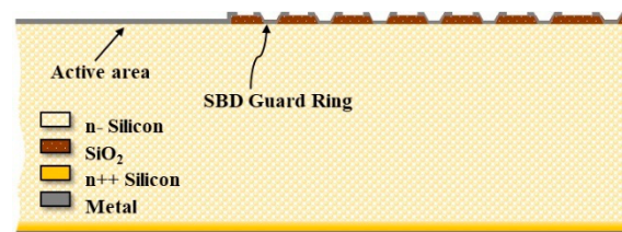
Figure 1. Simulation geometry, 2-D view of half-infinite and symmetric conventional SSBD structure consisting of a Schottky diode as the sensor surrounded with 7 guard rings.
